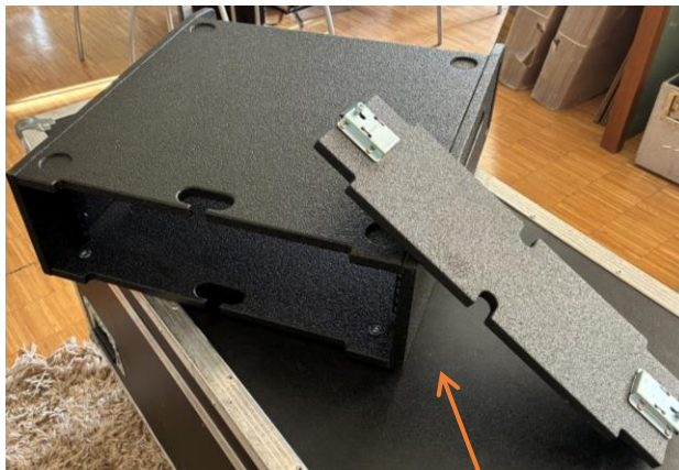
The CCU transport rack can be opened on the rear side to see connections
