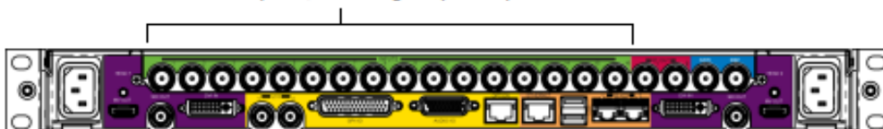
BNC connectors (16) for SD-SDI, HD-SDI, 3Gbps-SDI, and Analog Composite Inputs
