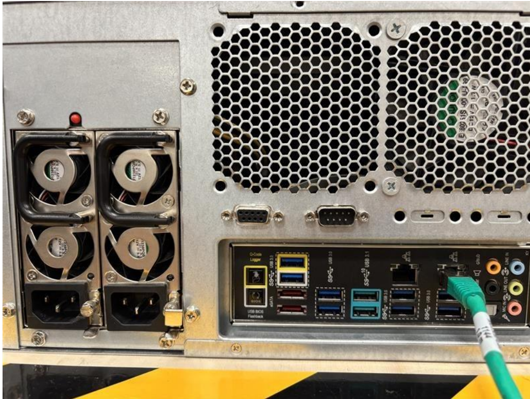
Rear system and computer I/O section
