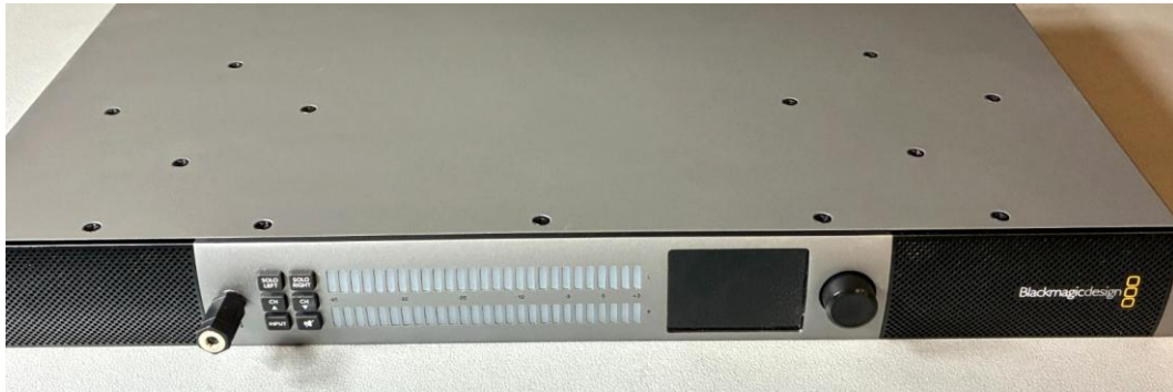
Front panel / LCD, level meters and monitoring controls
