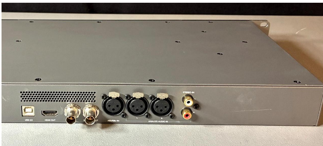
Rear connection detail / SDI, HDMI, AES/EBU, analog XLR and RCA
