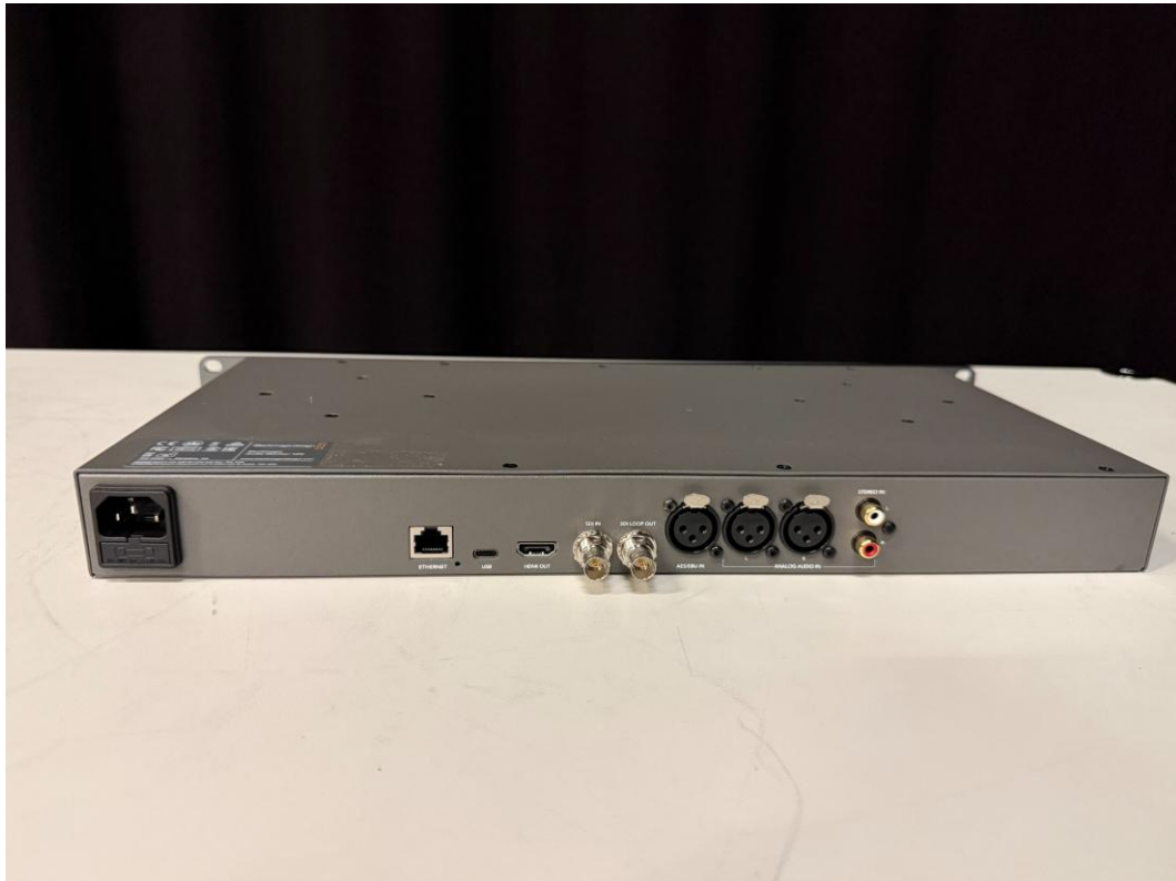
Rear panel / 10G Ethernet, USB-C, HDMI, 12G-SDI, AES/EBU, analog XLR and RCA
