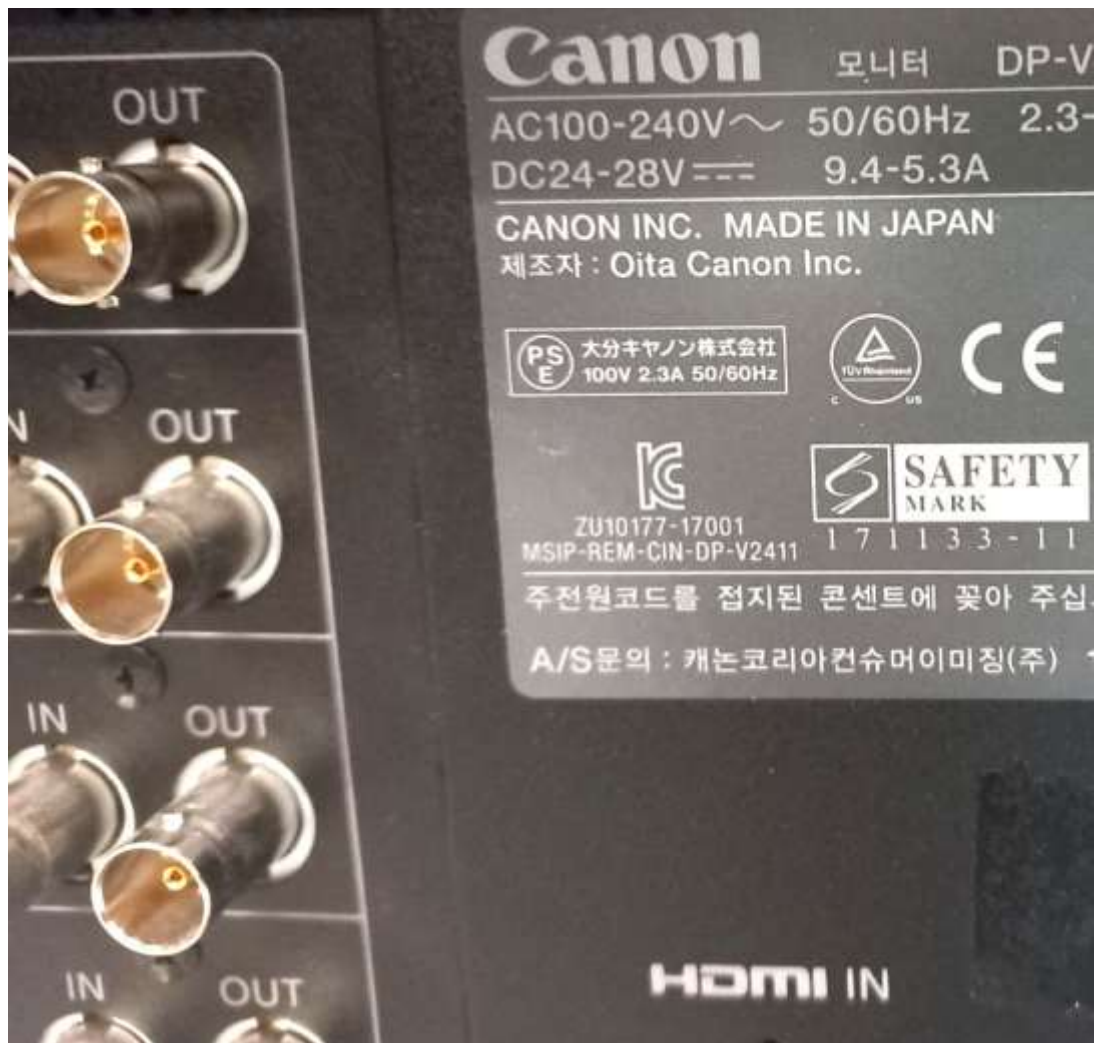
Rear connection detail with BNC connection area and HDMI input.
