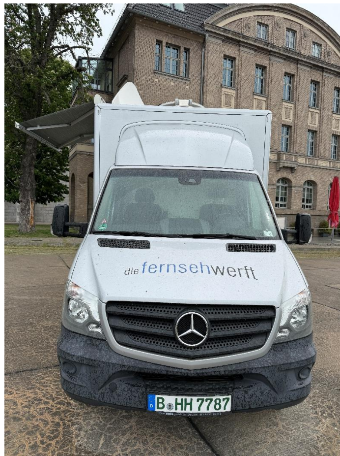
Used HD SNG Mercedes Sprinter 516 CDI prepared for 4x CCU controlled Cameras
