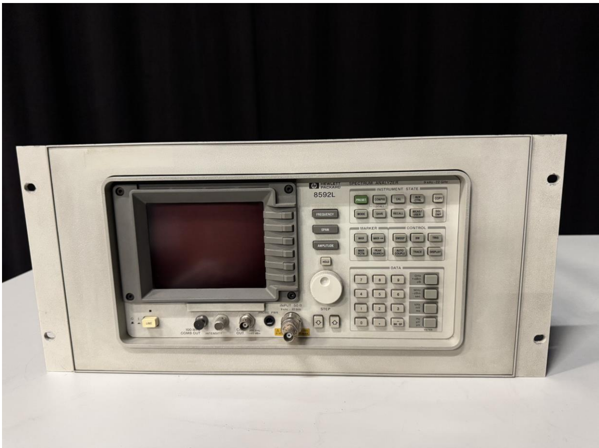
HP 8592L RF and microwave spectrum analyzer covering 9 kHz to 22 GHz in a rack-mount configuration.
