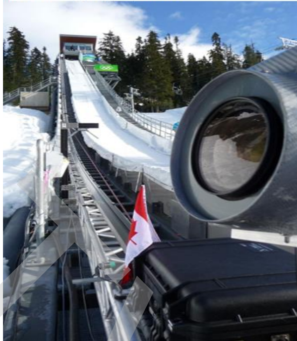
Railset 1 with bending rails and rail heating I.e. for ski jumping events
