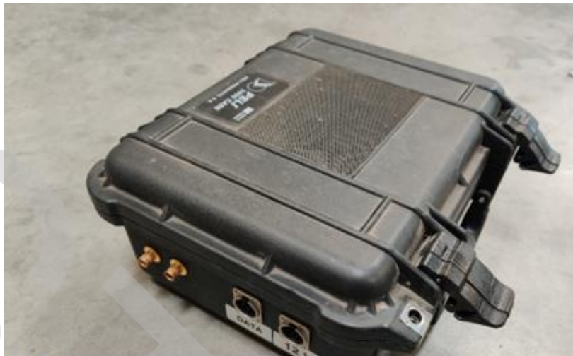
Peli case For power supply, audio/video cabling, data transmission, wireless equipment connections etc.
