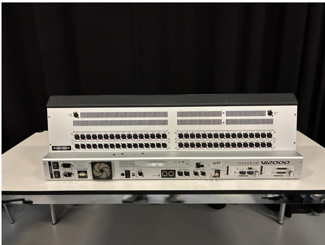
Rear overview with local I/O and console connection panels
