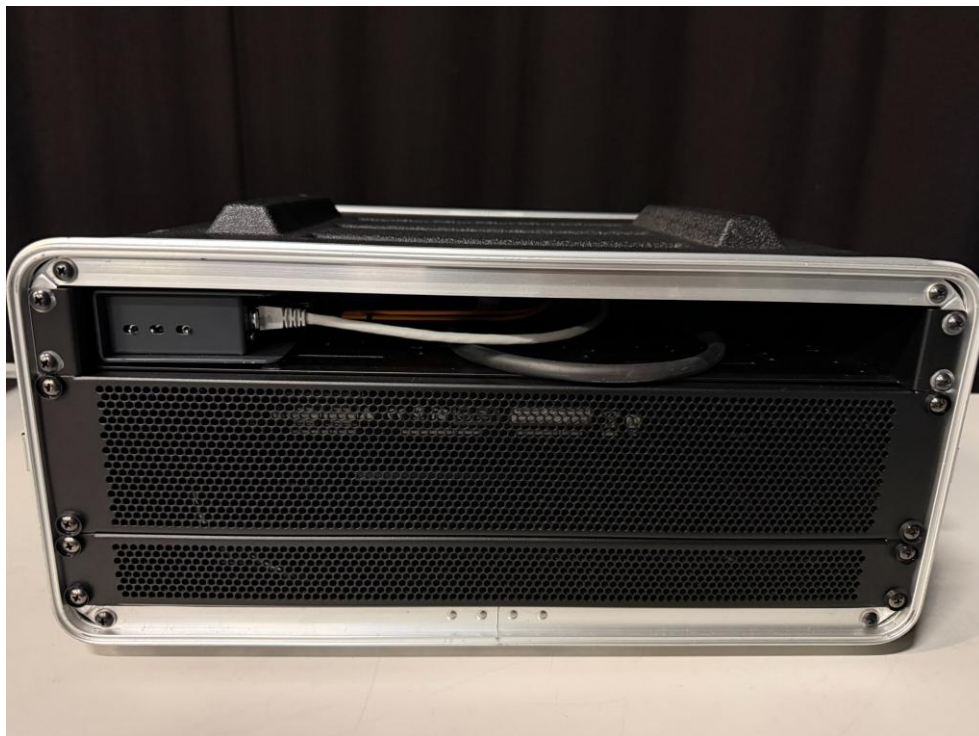
Stagebox installed in portable case with connected cabling
