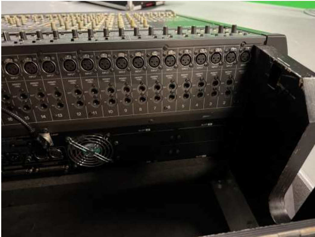
Rear input channel section with XLR inputs and insert points.
