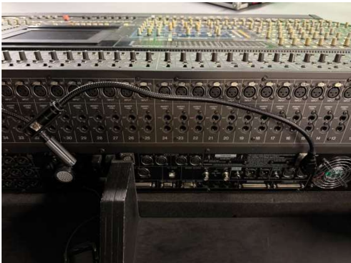
Rear I/O section with input channels, insert connections and control/digital audio connectors.
