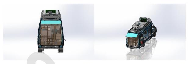
The back of the racks are accessible through two vertically operating doors. The bottom half folds down and provides secure footing area for the operators and the larger top half holds up providing sun and rain coverage during technical work.
