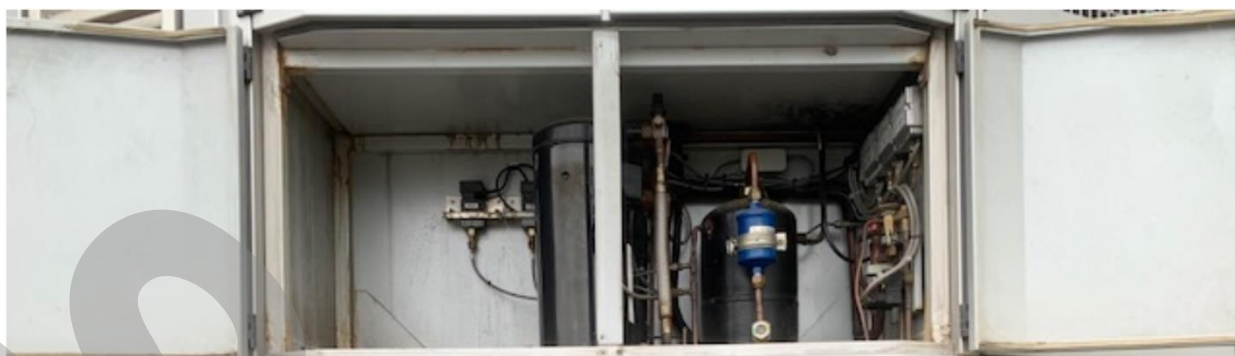
Front area - aircondition compressor + all connectors for the Tractor
